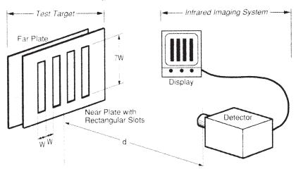
Note—A test pattern, consisting of four rectangular slots, permits a comparison of the temperature of the near plate of the test target with the far plate. The plates are initially at the same temperature. Someone increases the temperature difference between plates until an observer announces when the test pattern comes into view on the display. The difference in temperature at this point is the MRTD for that test condition.
