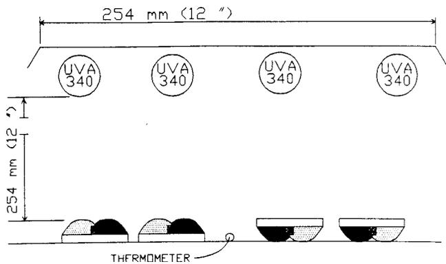
FIG. 2 UV Exposure Apparatus
