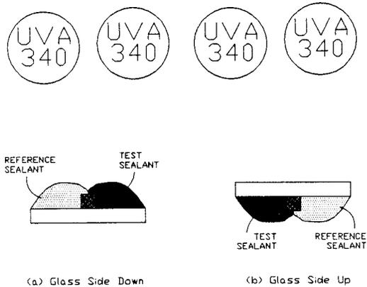
FIG. 1 Orientation of Test Specimen Under Lamps
