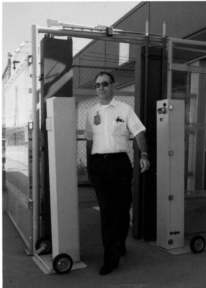
NOTE—Portable radiometric scanners are a new type of SNM monitor designed for temporary use. They are self-contained except for battery charging power and have wheels to make them portable.
