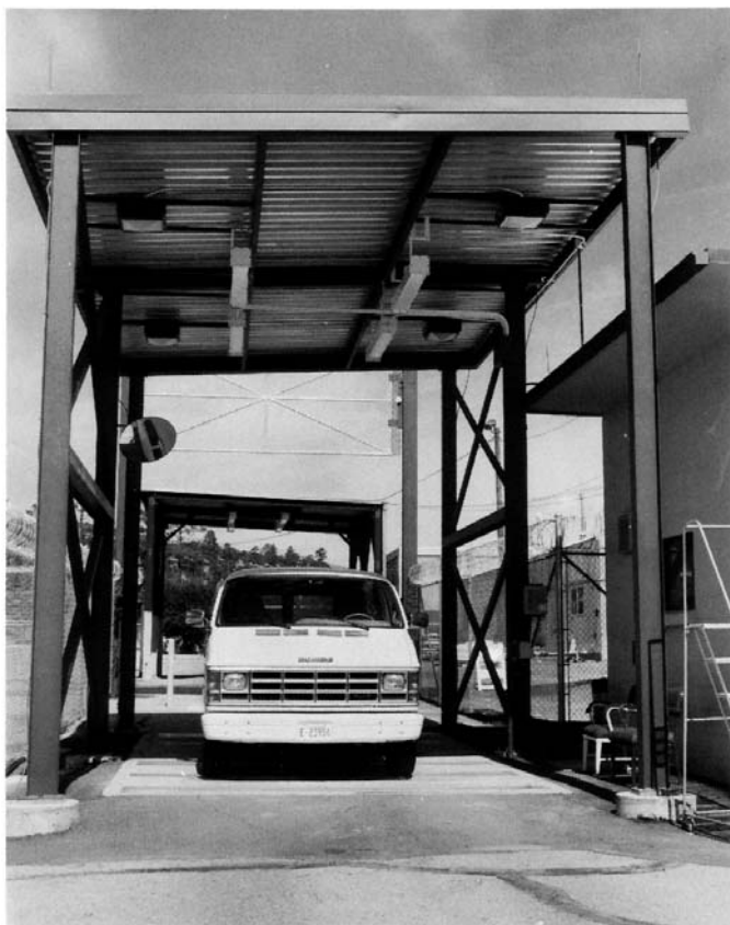
NOTE—Vehicle monitoring stations use an extended measurement time and have close proximity between detectors and vehicles, which makes them the most sensitive type of vehicle monitor.
