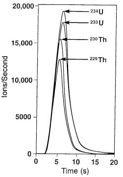
FIG. 3 Elution Profile for a Standard Containing 185 Bq/L (5000 pCi/L) <sup>229</sup>Th, 31 Bq/L (835 pCi/L) <sup>230</sup>Th, 18 Bq/L (500 pCi/L) <sup>233</sup>U, and 11 Bq/L (309 pCi/L) <sup>234</sup>U
