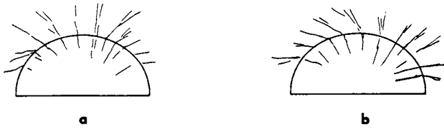
FIG. X1.6 Fine Hackle Lines may Change Direction at the Precrack Boundary
