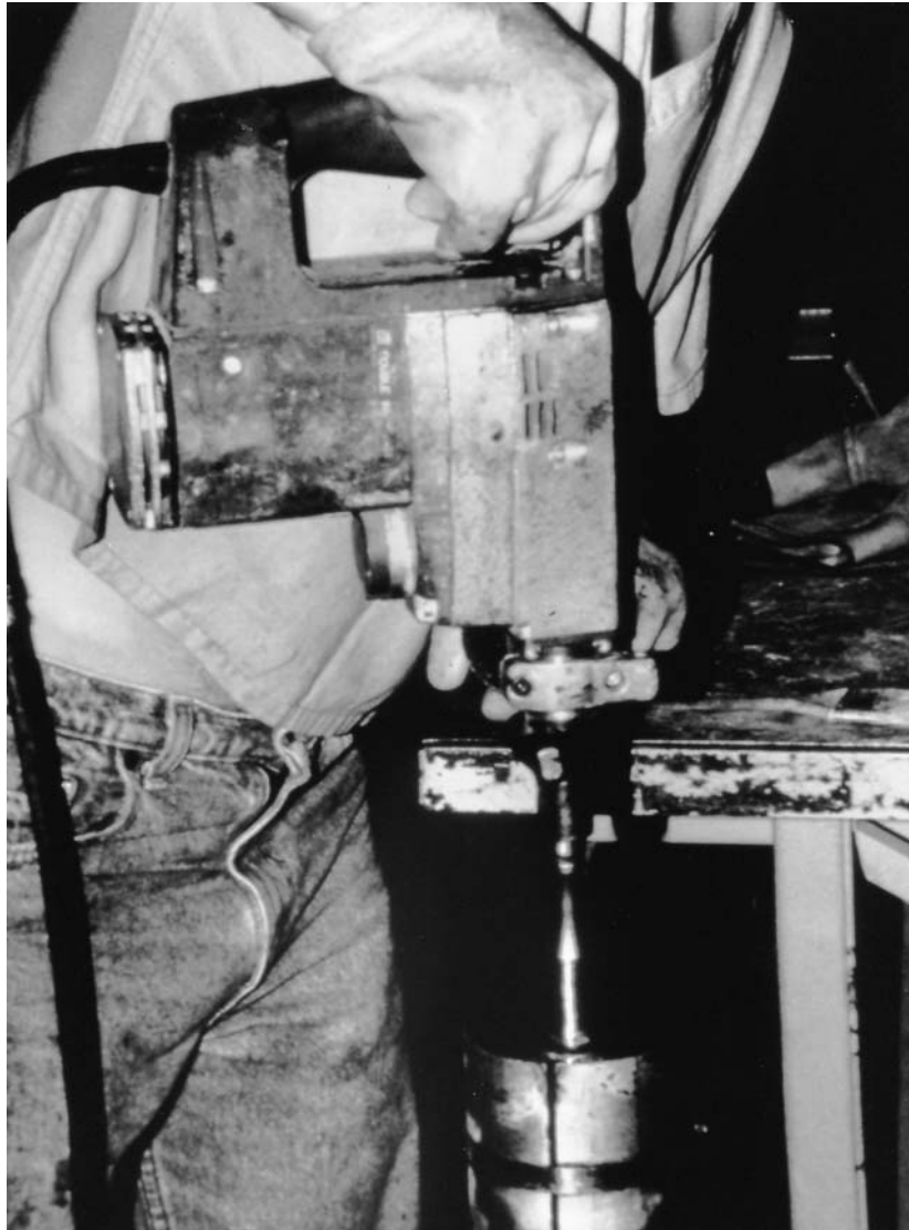
FIG. 1 Vibrating Hammer for Molding RCC Specimens
