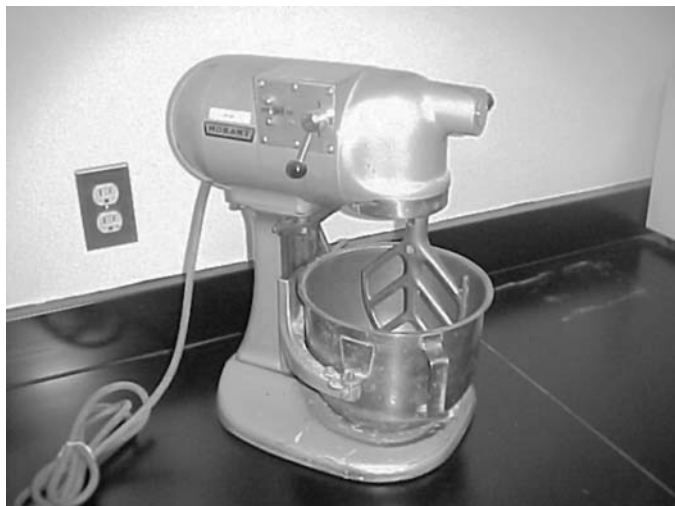
FIG. 2 Special Mixer for Castable Refractories
