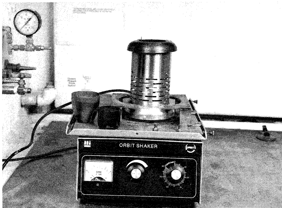
FIG. 1 Electric Bunsen Burner Mounted on the Orbital Shaker
