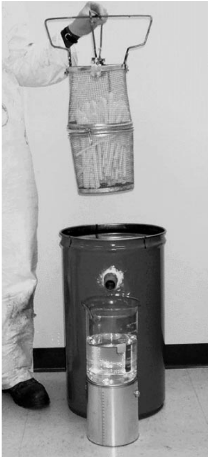
FIG. A1.2 Foam Beads In Cage Ready For Submersion In Water Tank
