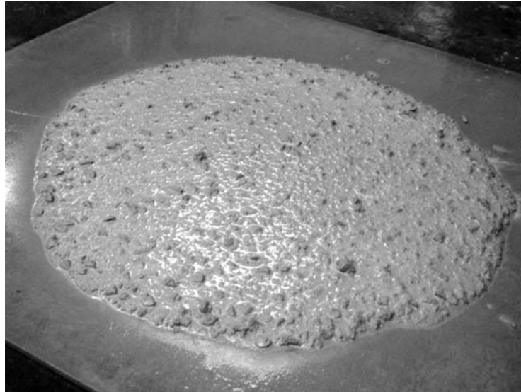
FIG. X1.2 VSI = 1 – Concrete Shows Slight Bleeding Observed as a Sheen on the Surface.
