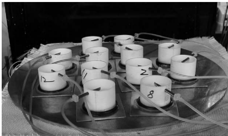
FIG. 3 Test Coupons on Hot Plate
