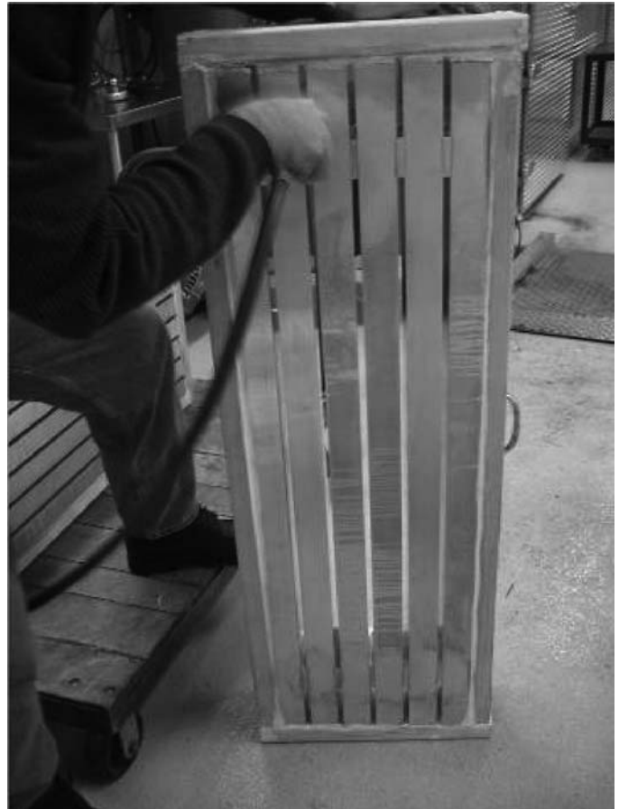
FIG. 1 An Assembled Test Jig Apparatus Ready for Joint Filling with a Perimeter Seal Applied in the Wood Test Buck
