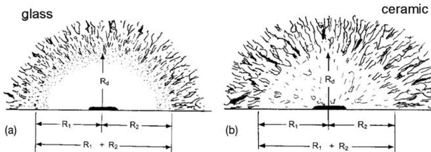
NOTE—(a) shows a schematic of such a mirror with the mist-hackle boundary marked in glass, and (b) shows a comparable image in a polycrystalline ceramic. The ceramic has some intrinsic microstructural roughness inside the mirror. The mirror-hackle boundary is marked. Use an average radius:  $R_{avg} = \{(R_1 + R_2 + R_d) / 3\}$ .
