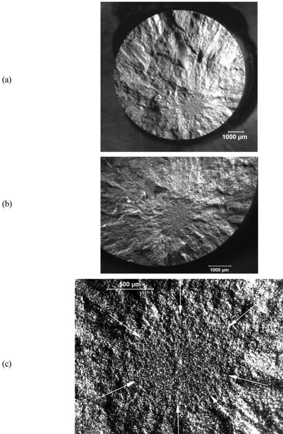
NOTE—Notice how clear the mirror is in the low power images in (a) and (b). The mirror boundary (arrows in c) is where systematic new hackle forms and there is an obvious roughness difference compared to the roughness inside the mirror region.
