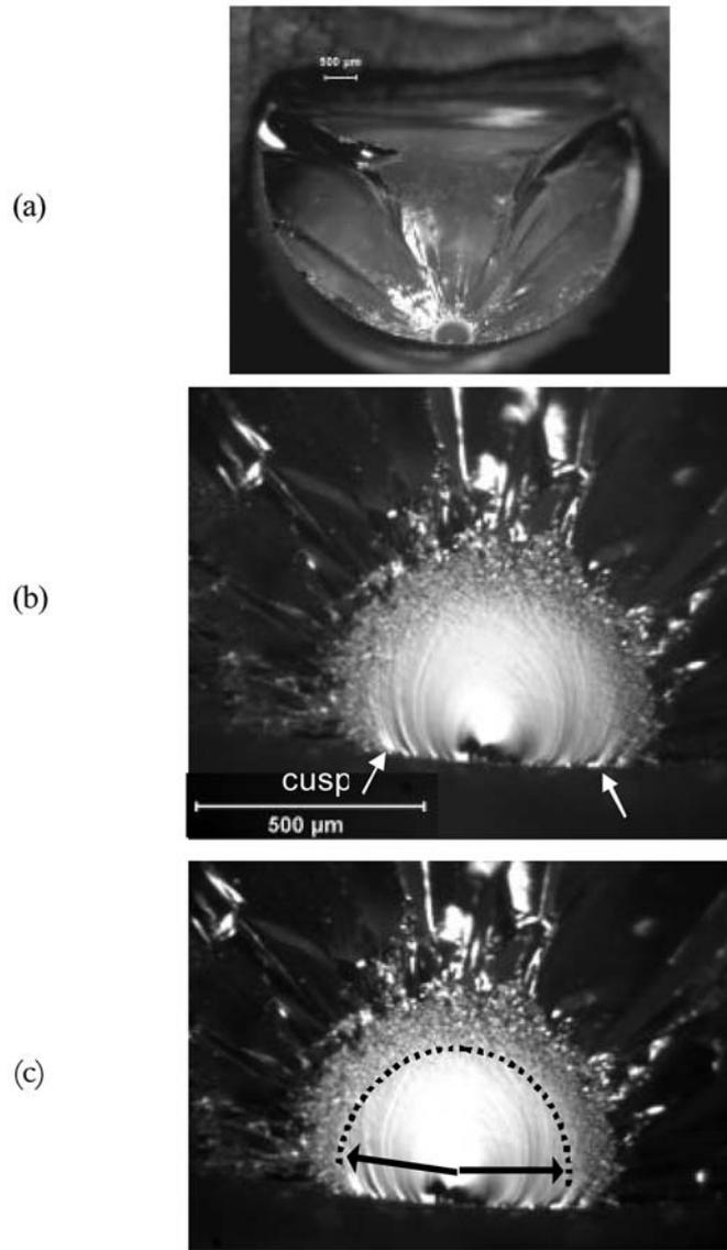
NOTE—Mirror measurements should not include the inward bend of the mirror and may be made as shown in (c).
