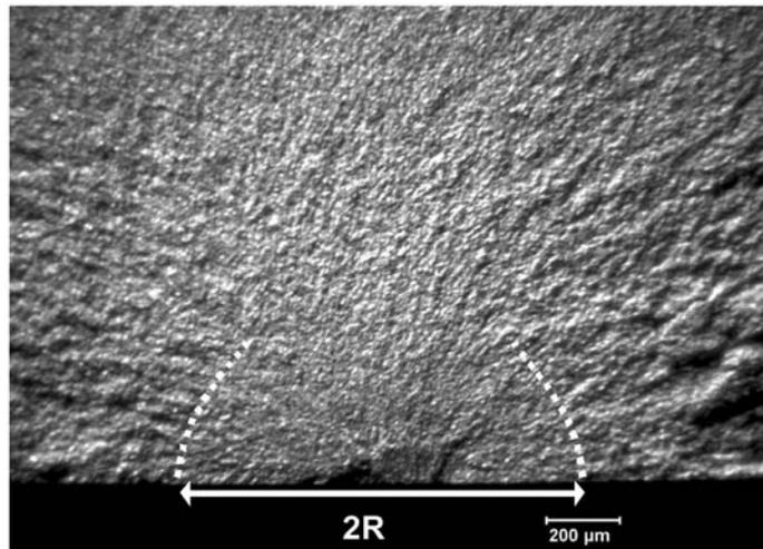
NOTE—The mirror is incomplete into the bend stress gradient, but the mirror sides can be used to construct boundary arcs in (c) [(b) and (c) are close-ups of (a)]. Radii are measured in the direction of constant stress along the bottom.
