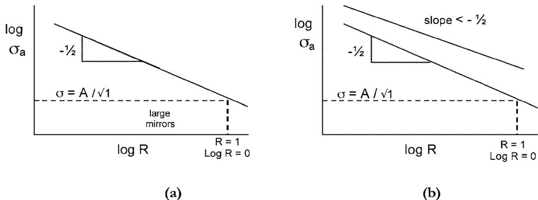
NOTE—Compressive residual stresses move the locus upwards as shown in (b), but with a different slope and intercept. Tensile residual stresses move the loci below the baseline curve (not shown).
