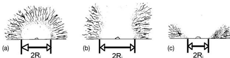
NOTE—If the mirror is small relative to the part size, then the mirror may be semicircular, as shown in (a). Weaker parts have larger mirrors that flare into the interior and are incomplete, as shown in (b) and (c). Measure the mirror size ( $R_1$  or  $2R_1$  for the mirror-mist in the illustrations here) in the direction of constant stress.
