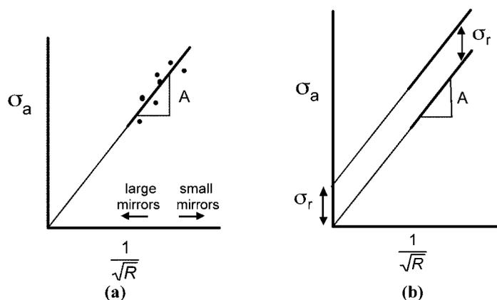
NOTE—(a) shows the trend for residual stress-free parts; (b) shows it for parts with residual stresses. Compressive residual stresses move the locus up with a positive intercept  $\sigma_r$ , but with the same slope. Tensile residual stresses shift the data downwards with a negative intercept (not shown).
