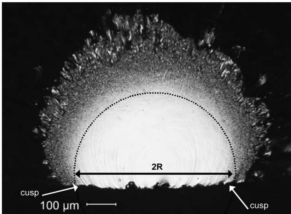
NOTE—Fracture mirrors centered on surface origins in glass have inward tilting cusps. These should be truncated and a mirror site measured by using the arc of the overall mirror shape. This mirror is slightly elongated into the interior due to a bending stress gradient.
