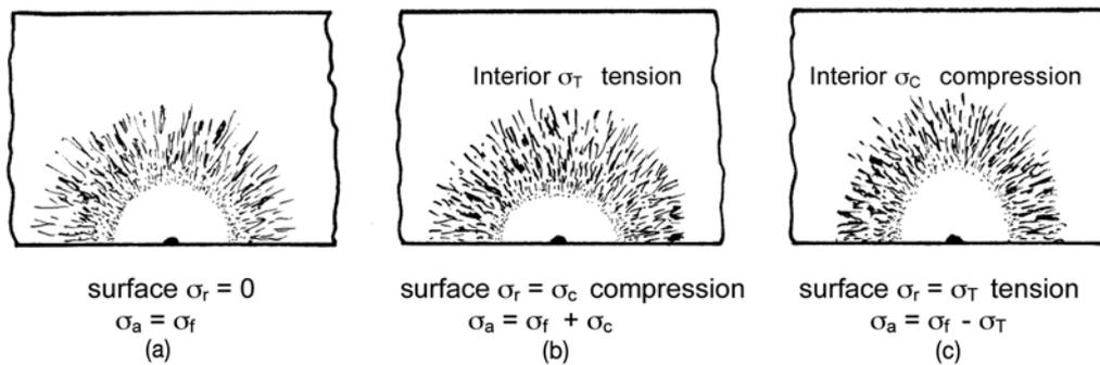
NOTE— $\sigma_a$  is the applied stress to cause fracture, and  $\sigma_f$  is the fracture stress in an annealed plate in tension. (a) shows a surface mirror in an annealed plate. (b) shows the mirror shape in a plate with surface compression stresses that decrease into the interior and become tensile. (c) shows a mirror in a plate with surface tensile stresses that diminish into the interior and become compressive.
