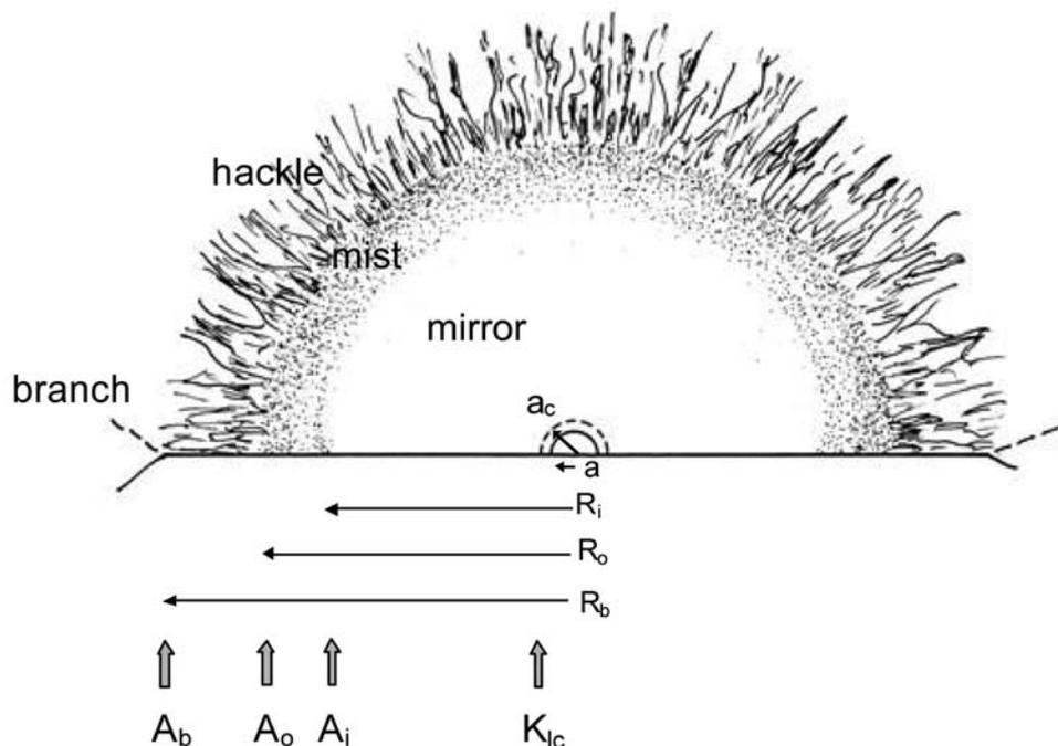
NOTE—The initial flaw may grow stably to size  $a_c$  prior to unstable fracture when the stress intensity reaches  $K_{Ic}$ . The mirror-mist radius is  $R_i$ , the mist-hackle radius is  $R_o$ , and the branching distance is  $R_b$ . These transitions correspond to the mirror constants,  $A_i$ ,  $A_o$ , and  $A_b$ , respectively.
