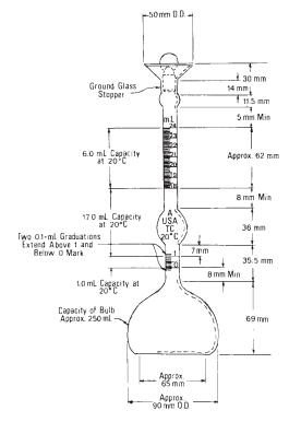
Note-Variations of a few millimetres in such dimensions as total height of flask, diameter of base, and so forth, are to be expected and will not be considered sufficient cause for rejection. The dimensions of the flask shown in Fig. 1 apply only to new flasks and not to flasks in use which meet the other requirements of this test method.
