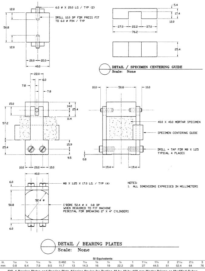
FIG. 1 Bearing Plates and Bearing Plate Aligning Device for Testing 40 by 40 by 160-mm Mortar Prisms as Modified Cubes
