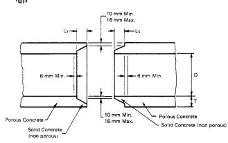
NOTE—See Tables 1 and 2 for values of D, T, and L<sub>a</sub>. FIG. 1 Joint Dimensions
