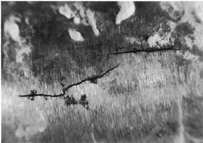
FIG. 2 Typical External Stress Corrosion Cracks (5× Magnification)
