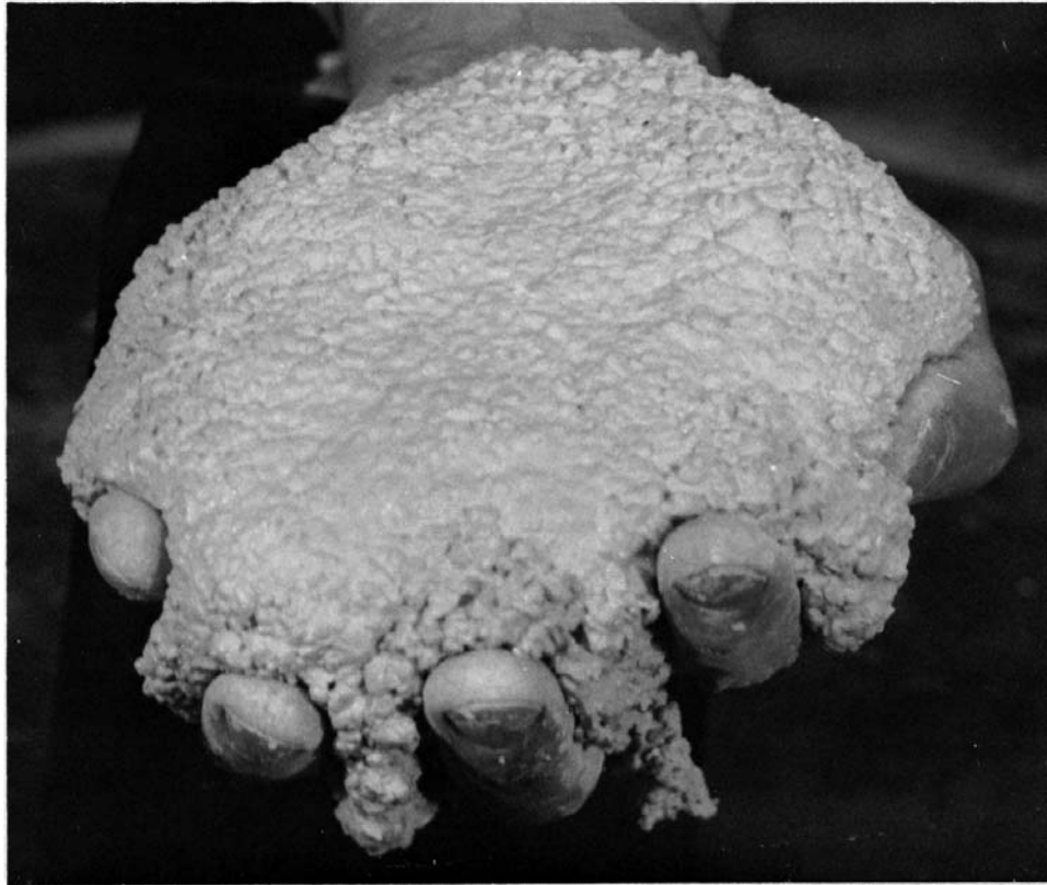
FIG. 2 Range in Consistency of Castable Mixes as Shown by Ball-in-Hand Tests
