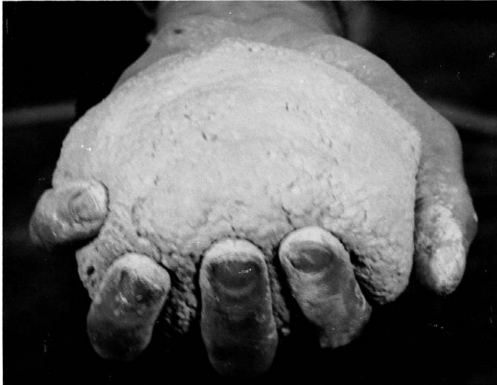
FIG. 4 Range in Consistency of Castable Mixes as Shown by Ball-in-Hand Tests
