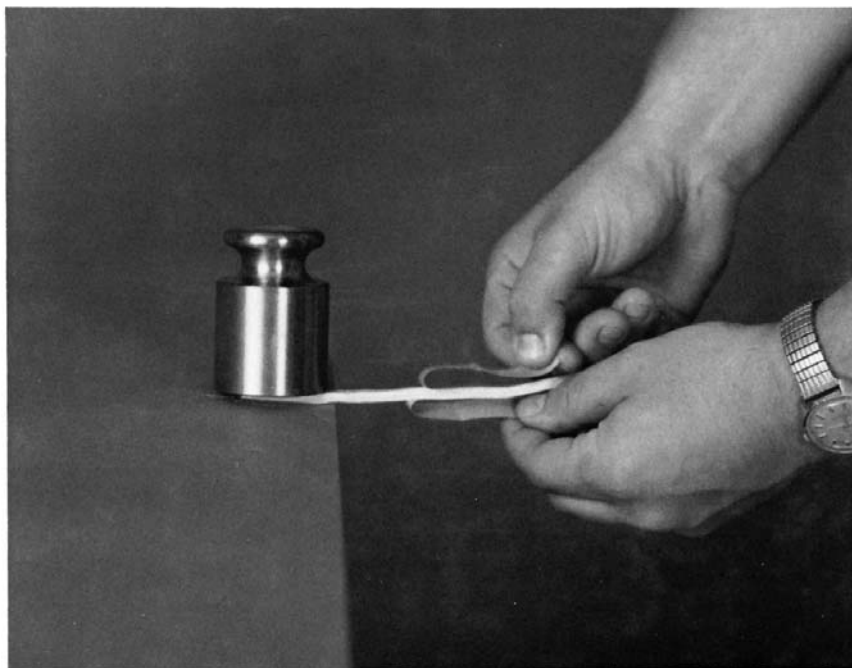
FIG. 1 Release Paper Peeling Procedure
