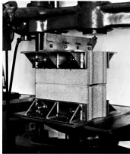
FIG. 8 Concrete Block Test Assembly Positioned in Testing Machine
