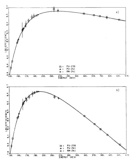
Note 1—(a)—Typical relative efficiency curve for 2 kg aged plutonium-oxide sample. Relative spectral intensities for <sup>239</sup>Pu, <sup>241</sup>Pu, and <sup>241</sup>Am are used to generate response function. Vertical scale is natural logarithm of relative units. A300 mm<sup>2</sup> by 7 mm planar Ge detector was used for the spectral measurements.
