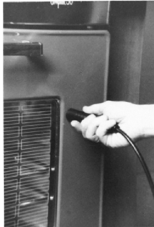
FIG. 4 Applying the Thermesthesiometer to a Vertical Surface
