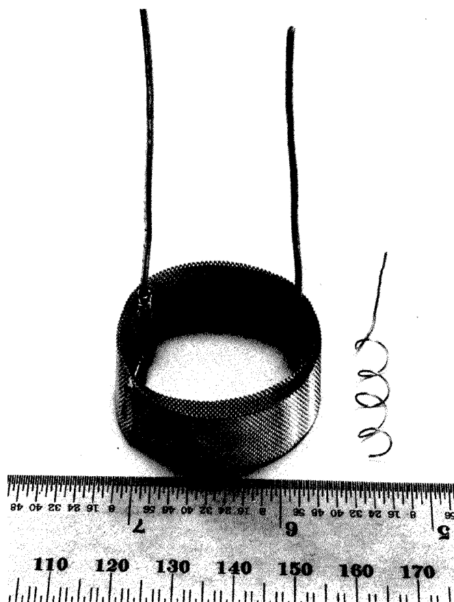
FIG. 2 Working Electrode (Top View)
