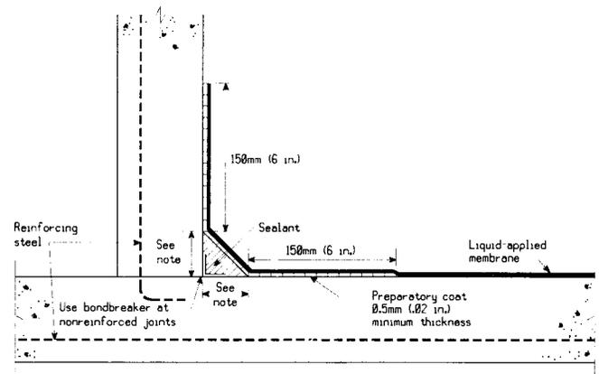
NOTE 1—Dimension shall be 25 mm (1 in.) for a nonreinforced butt joint (movement between 1.6 mm (0.063 in.) and 3.2 mm (0.125 in.)) or 13 mm (0.5 in.) for a reinforced joint as shown (movement less than 1.6 mm (0.063 in.)).
