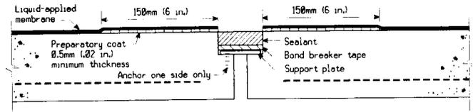
FIG. 8 Typical Expansion Joint (see 10.4.4.3 and 14.5.6)
