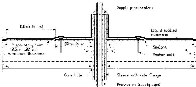
**FIG. 3 Termination at a Core-Drilled Sleeve Having a Wide Flange**
