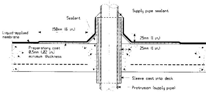
**FIG. 2 Termination at Cast-in-Place Sleeve (Protrusion Installed)**
