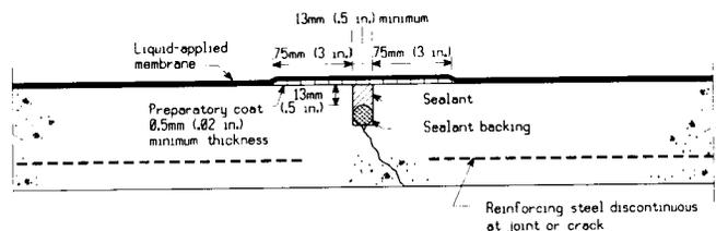
**FIG. 5 Treatment of Nonreinforced Cracks and Joints** (see 10.4.4.2 and 14.5.3)
