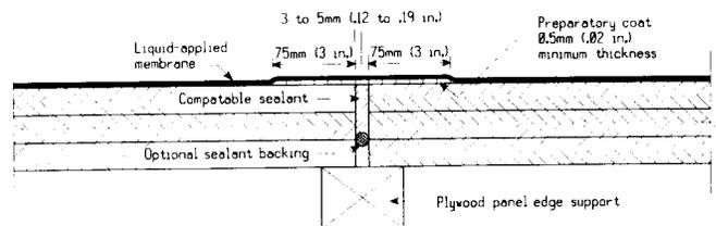
FIG. 6 Treatment of Plywood Panel Joints (see 8.5.1 and 14.5.4)
