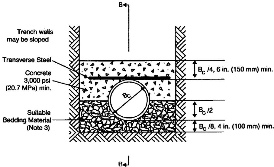
Load Factor: 3.4 Reinforced Concrete  $p = 0.4\%$
