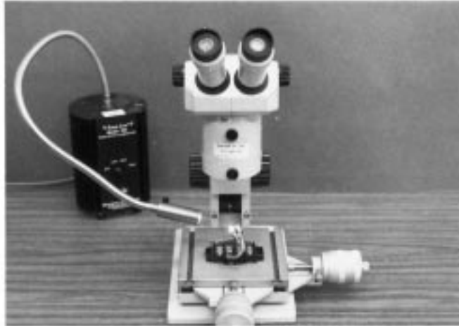
FIG. X4.1 Binocular Stereomicroscope with Directionally Adjustable Fiber-Optical Light Source and Variable Magnification Between 5 and 80 \times .
