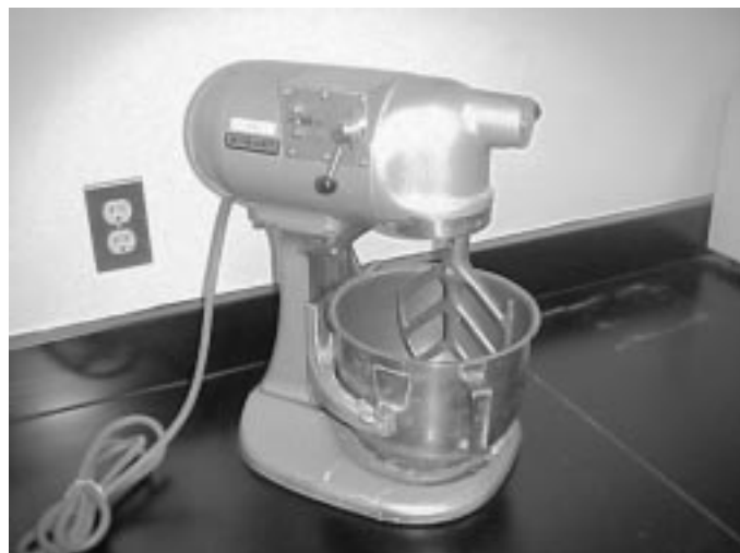
FIG. 1 Special Mixer for Castable Refractories
