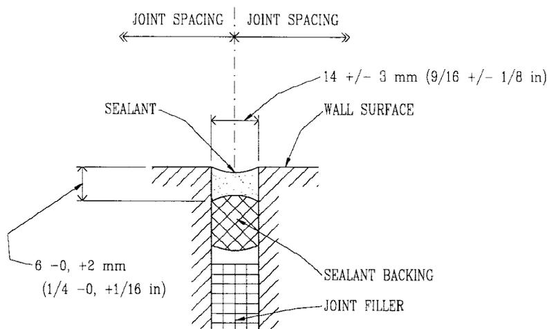
**FIG. 9 Cross-Section of a Typical Butt Sealant Joint**
