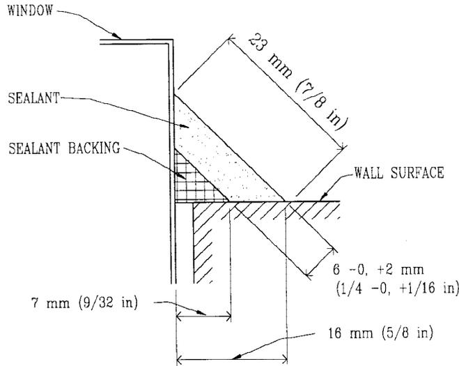
FIG. 10 Cross-Section of a Typical Fillet Sealant Joint
