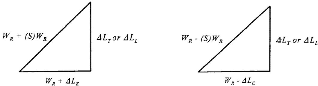
FIG. 8 Sealant Joint Movement Combination
