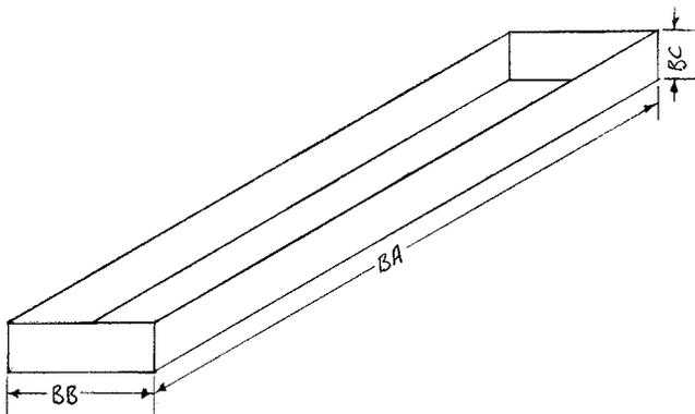
NOTE 1—*Hardware Description for Specimen Tray* in Figs. 2-4. Open top box 0.16 mm (0.024 in.) thick (22–26 US standard gage) stainless steel sheet with the vertical edges of the box overlapped not to exceed 7 mm (0.273 in.) in seam width, and joined to be watertight.
