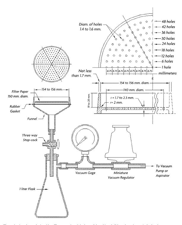
Note—The gasket is to be synthetic rubber. The stopcock and the bore of the tubing shall be at least 4-mm. A check valve or water trap, or both, is suggested for the connection to the vacuum source.
