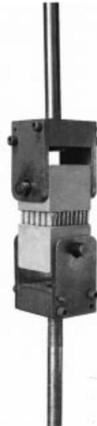
FIG. 1 Flatwise Tension Test Setup
