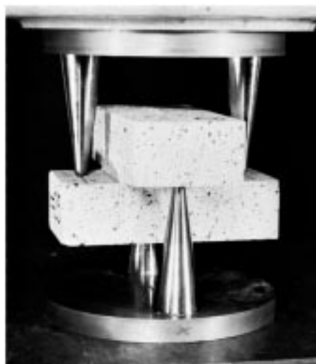
FIG. 4 Cross-Brick Specimen Mounted on Special Fixture
