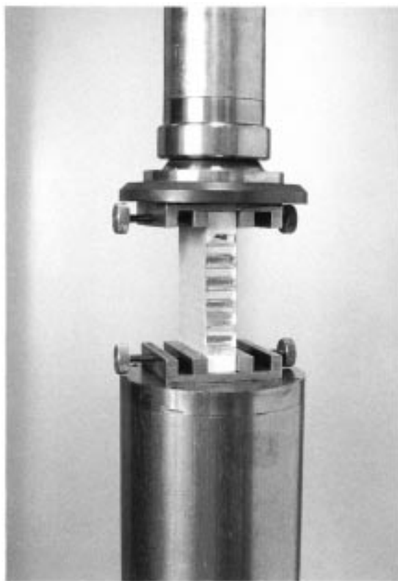
FIG. 1 Edgewise Compression Test Setup
