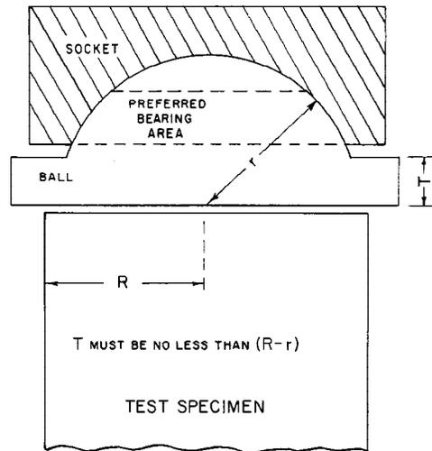
NOTE—Provision shall be made for holding the ball in the socket and for holding the entire unit in the testing machine.
