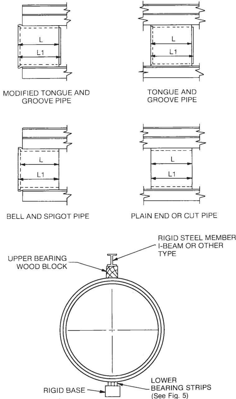
NOTE 1—The figures illustrate a method of applying the load to the pipe.
