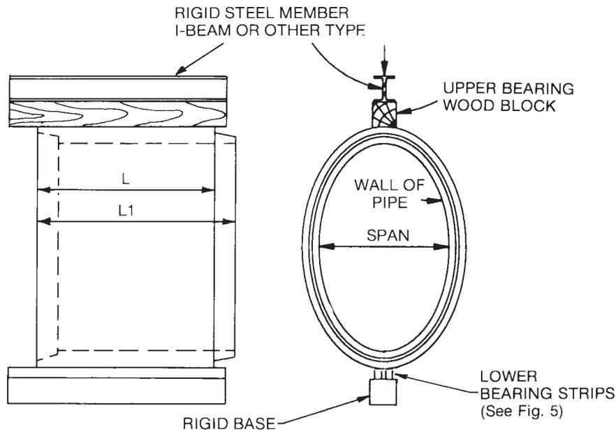
NOTE 1—The figure illustrates a method of applying the load to the pipe.
