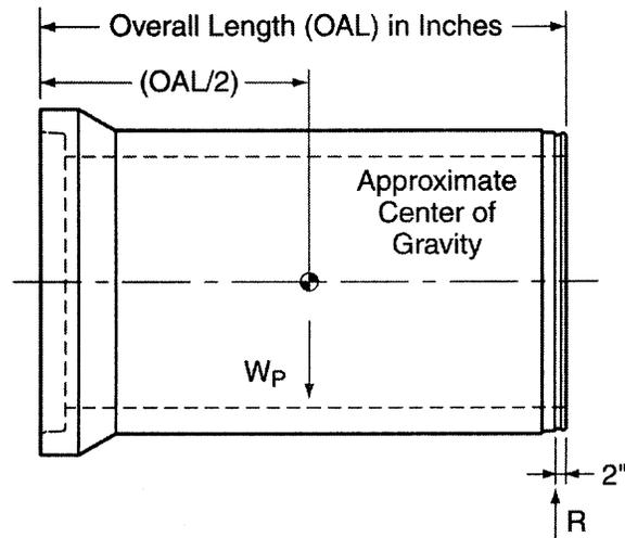
FIG. 10 Simplified Center of Gravity of Pipe
