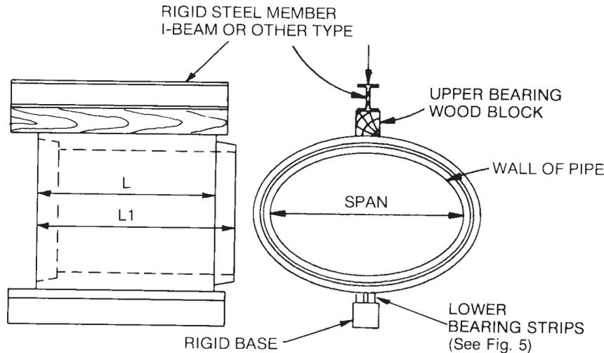
NOTE 1—The figure illustrates a method of applying the load to the pipe.
