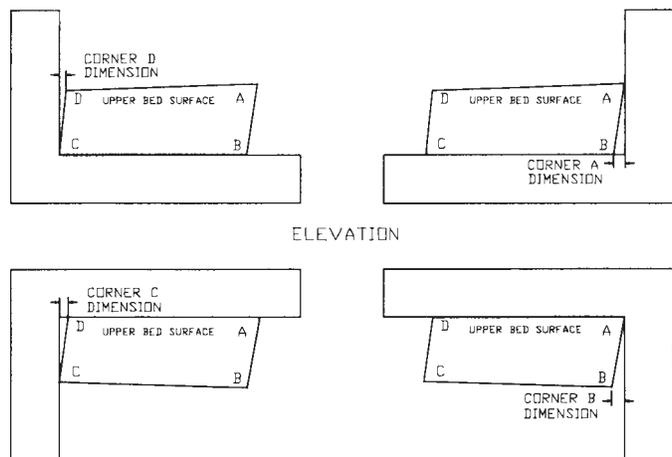
FIG. 4 Out-of-Square Measurements
