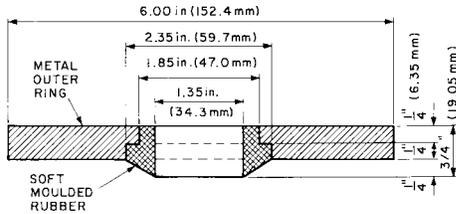
NOTE 1—The outer ring is a steel disk approximately 6 by 1/2 in. (152 by 13 mm), weighing approximately 3 1/2 lb (1.58 kg).
