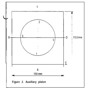
Measure the distances from the centre of each top edge of the lower auxiliary platen to the nearest point on the bottom edge of the device and adjust the position of the device until the differences between pairs of measurements from opposite edges of the platen to the device do not exceed 0.10 mm.
