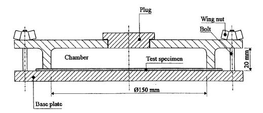
Fig.1 - Exposure framework for elastomers to injection products (dimensions in mm)
