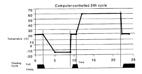
Figure 1 - Thermal cycling between -15  $\pm$  2°C, 20  $\pm$  2 °C and 60  $\pm$  2 °C
