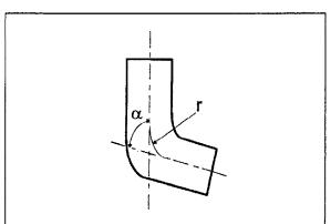
Figure 1. Illustration of radius 'r' and angle 'a' bend
