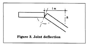
Minimum shear load values in the joint shall be  $10 \text{ N} \times \text{DN}$ .
