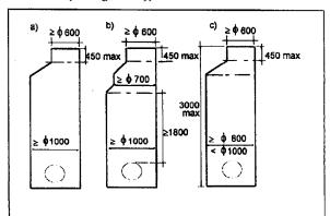
Figure 2: Examples of circular manholes
