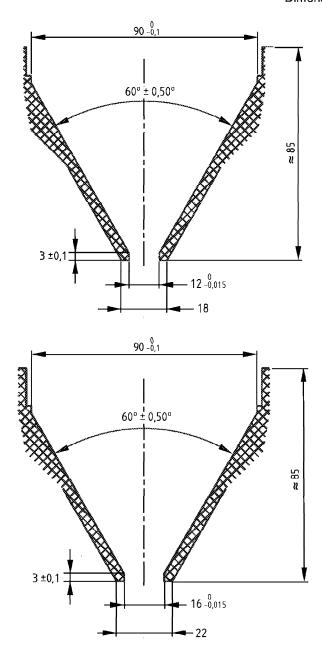
Figure 3 — Additional funnels for flow unit for fine aggregate
