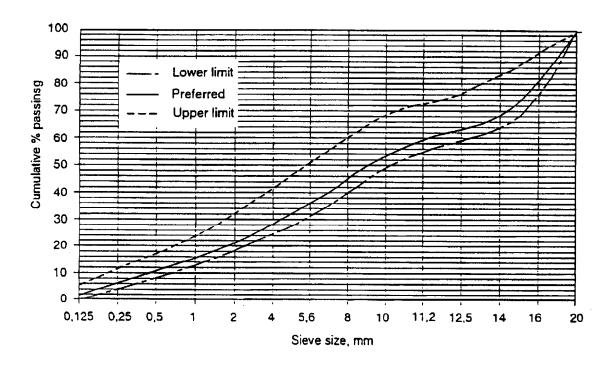
Figure 1: Grading limits for aggregate in concrete prisms
