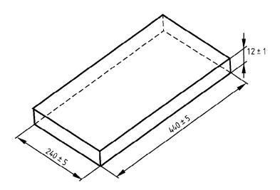
Figure 1 — Metal test plate
