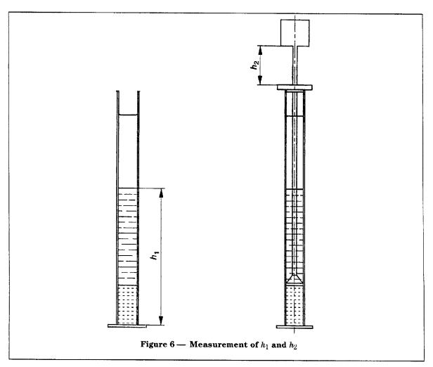
Locate the collar on top of the cylinder and then lock it onto the plunger rod.
